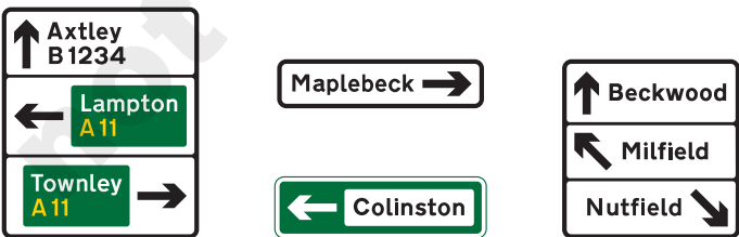
Examples of stack-type signs. Arrows indicate the direction of exits from the junction ahead; each is shown on a separate part of the sign. The ahead direction may not be shown for a junction with a minor side road
