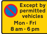
Repeater sign within a loading area
