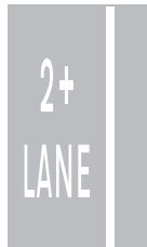
HOV lane road marking
