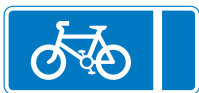
Mandatory with-flow pedal cycle lane. Hours of operation may be shown. Vehicles must not be driven or parked in this lane during its times of operation
