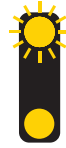
Lights warning of children likely to be crossing the road on their way to or from school (used with 'school' sign)
