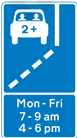
Start of HOV lane (near-side)
