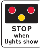
Plate used with level crossing warning signs: advance warning of light signals at a level crossing with or without a gate or barrier
