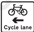
Pedal cycle lane on road at junction ahead or (where 'lane' is varied to 'track') cycle track crossing road at junction ahead
