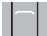
Stop line for trams at traffic signals where that part of the road is not used by other vehicles
