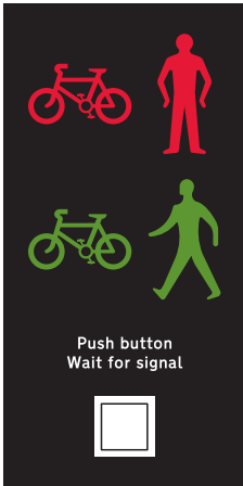
Near-side signals for toucan crossing
